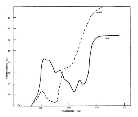
Figure 1: Light transmission through a single thickness of Solar Screen "Pink" (solid line) and "Amber" (broken line, afte<sup>-</sup> Sutton and Zimmerman, 1979). Measured with a Cary recording spectrophotometer model 14, Chemistry Department, Brookhaven National Laboratory.
