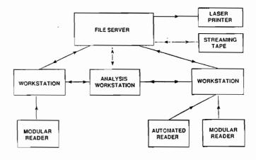
Figure 1. Network Schematic
