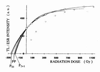
Figure 3. Regression on a simulated test curve 1/1, with 5% standard deviations on intensities; preset palaeodose (PP): 300 Gy; maximal dose taken into account on 1st DRC: 960 Gy.  $P_{S1}$ ,  $P_{2+1}$ : as in fig.2, the most probable value (the value obtained without errors). EF: exponential fit on 2nd DRC, using mean points. Dashed lines: ten first curves calculated with S1; solid lines: ten first calculated curves with 2+1.
