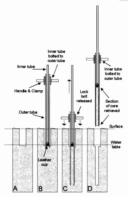
Figure 1. Basic parts of the Van der Staay suction-corer, as well as the working principles (adapted from van de Meene et al., 1979).
