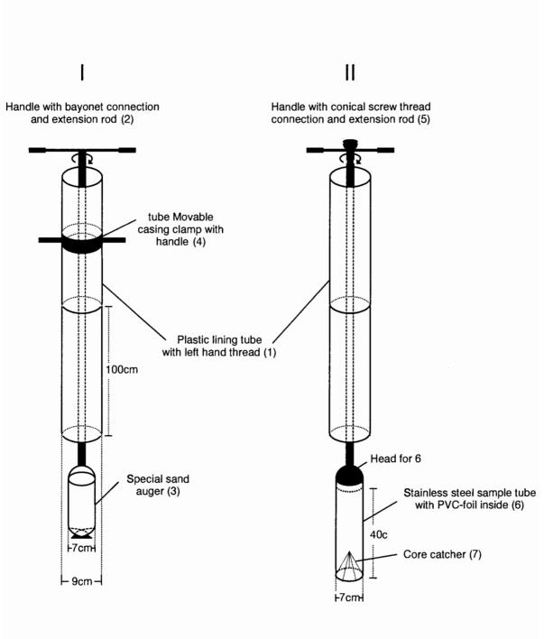
Fig. 1: Schematic drawing of the coring equipment
