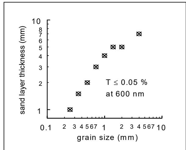
**Figure 3.** Sand layer thickness required to reduce the transmittance of 600 nm incident light to 0.05 % or less (the lower limit of the instrument used is 0.05 %) for the 8 largest grain-size classes tested.
