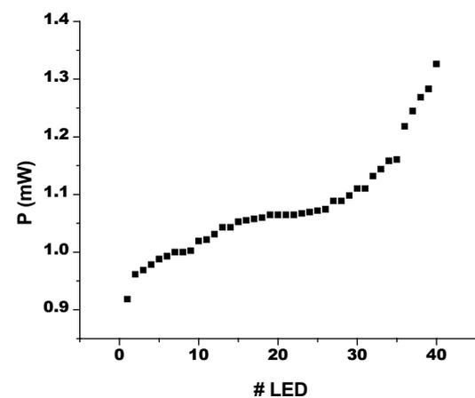
**Figure 12:** Power output of the 40 LEDs employed in the stimulation unit.
