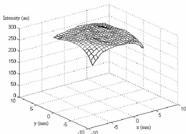
**Figure 13:** Measured illumination pattern in the sample plane.
