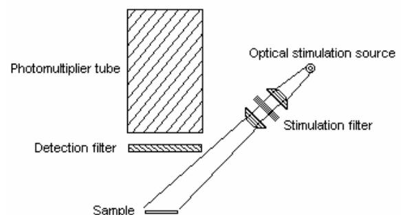
**Figure 1:** Standard configuration of a photoluminescence reading system
