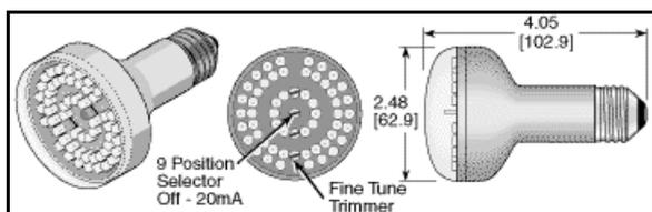
**Figure 3:** Format of the adjustable screw-base, colored LEDtronics darkroom safelight bulbs. The dimensions are in inches and mm (parentheses) (image from [www.ledtronics.com](http://www.ledtronics.com)).
