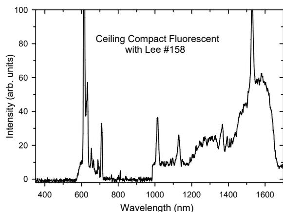
**Figure 1:** Spectrum from a filtered (Lee #158) compact fluorescent ceiling lamp, mounted in a reflector-floodlamp configuration (Lumatech Lighting, Model 1051x for 5W compact fluorescent bulbs, [www.lumatechlighting.com](http://www.lumatechlighting.com)), showing the typical Hg emission lines superimposed on a fluorescent-lamp emission continuum.
