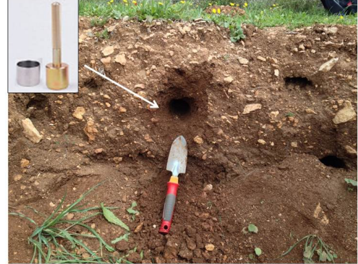
Figure 1. A typical soil profile of one of the pits in Har-Eitan. The holes in the profile represent the locations where undisturbed soil or other samples were taken. Insert: The sampling ring and ring holder used to take the undisturbed samples.
