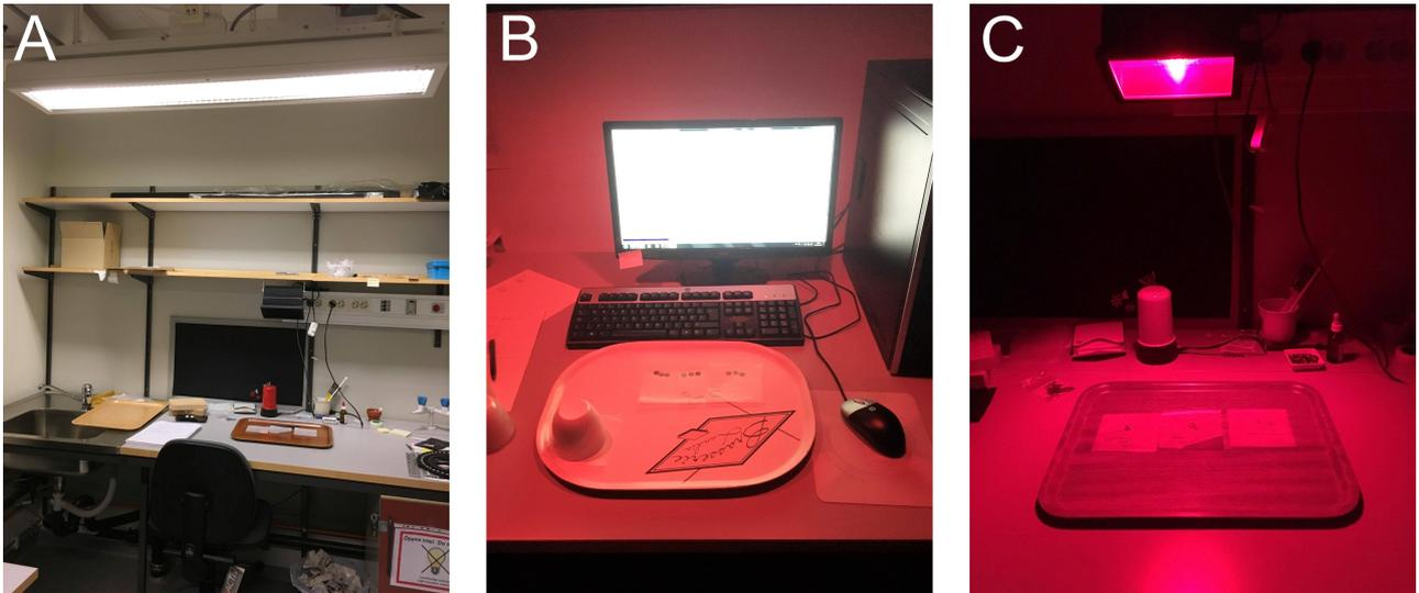
Figure 1. Indoor experiments. A. In experiment I-1, the samples were exposed to light from a fluorescent tube for 10 s to 15 min. B. In experiment I-3, samples were placed in front of a computer screen for 10 s to 15 min. C. In experiment I-4, the samples were exposed to red, darkroom light for 24 hours.
