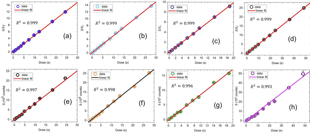
Figure 8. Test dose corrected (upper row) and uncorrected (lower row) dose responses of  $Al_2O_3:C$  irradiated with wine glass attenuator (a and e), microscope coverslip glass (b and f) PTFE (c and g) and ABS (d and h). Each data point represents the average and standard error for 3 dosimeters. The adjusted  $R^2$  is also represented to show the goodness of the fit
