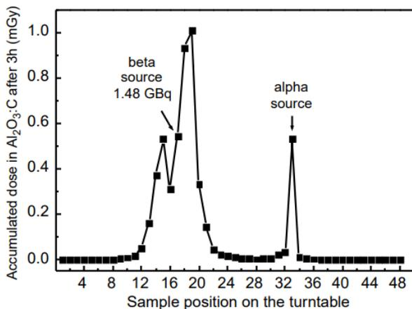
Figure 1. Accumulated dose due to leakage radiation in 3 h at various carousel positions in a Risø TL/OSL-DA-15 reader measured with  $\text{Al}_2\text{O}_3:\text{C}$  dosimeters, with both beta and alpha sources installed. The position underneath the beta source indicated on the plot is not the position of maximum dose. The position under the alpha source is also a hotspot as indicated on the plot (Fig. 4. from [Kalchgruber et al. \(2002\)](#))
