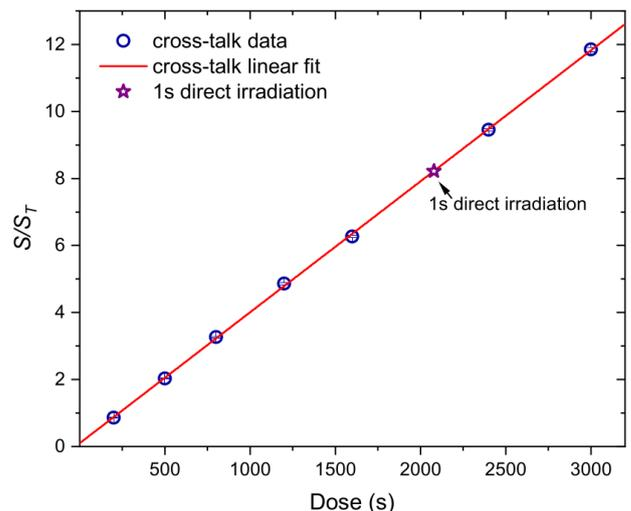
Figure 6. Reference dose–response curve of  $\text{Al}_2\text{O}_3:\text{C}$  dosimeter built up with the  $\beta$ -source of the Risø reader (Risø TL/OSL-DA-20) using cross-talk for indirect irradiation. The red line indicates the linear fit of the irradiation cross-talk  $S/S_T$  vs. equivalent dose data while the purple star symbol represents the 1s direct irradiation data.
