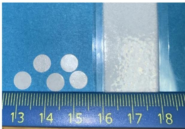
Figure 2. OSL Luxel<sup>®</sup> round punch-out and tape. The round punch-out was obtained by using a hole punch on the tape. The thickness of the dosimeter is 0.3 mm and diameter is 6.0 mm.
