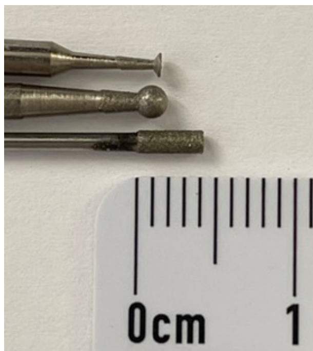
Figure 1: A (top): 1.5 mm diamond disc burr drill bit; B (middle): 2 mm diamond ball burr drill bit; C (bottom): 1.5 mm diamond core drill bit; all three drill bits are used in the extended MET sampling protocol.
