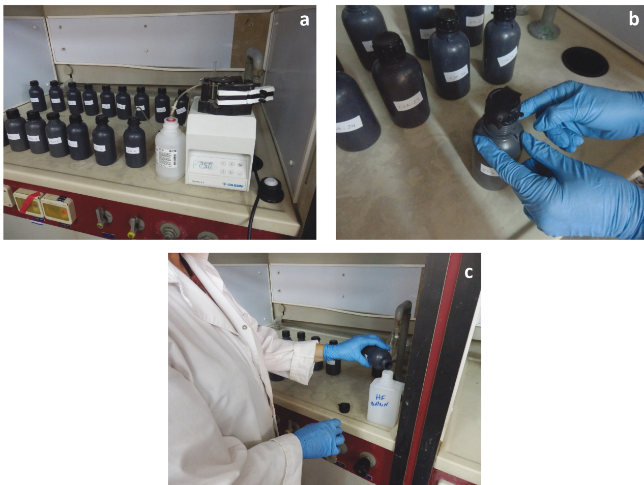
Figure 1. Setting of the HF etching procedure within a chemical fume hood. a) The HF is transferred from the HF bottle to the sample bottles through the peristaltic pump. The cup connected to the pump tube (sample closest to the pump) is moved from one sample to the next. b) The bottle cap that is moved from sample to sample has two holes, one with the exact diameter of the tube, where it is placed, and a smaller one to release air. c) After 40 minutes of soaking, the spent acid is carefully poured into a waste bottle. Note that the sample will settle in the shoulder of the bottle.
