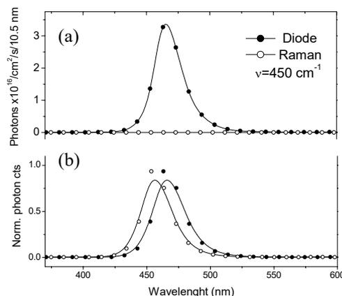
**Figure 2:** a) Measured blue light photon spectrum (derived from figure 1) and the calculated Raman scattering spectrum (for assumed single emission line and an efficiency of 10<sup>-7</sup> at each excitation wavelength) using a Raman shift of 450 cm<sup>-1</sup> for quartz. The photon flux was calculated for an integral intensity of 50 mW.cm<sup>-2</sup>. b) Data from a) plotted after normalisation by the peak counts.
