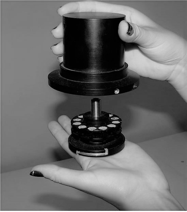
Figure 3. The sample holder, hosting up to 24 discs (below), and the container.
